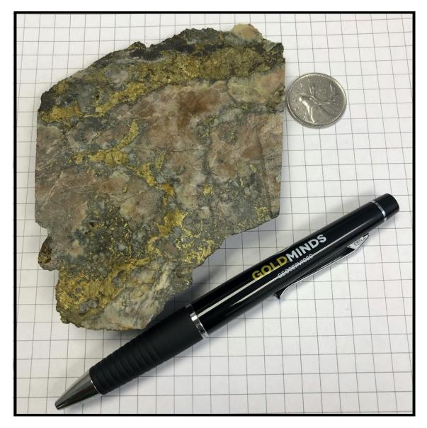
Figure 2. Sulphide mineralization from channel sample on B2 property
