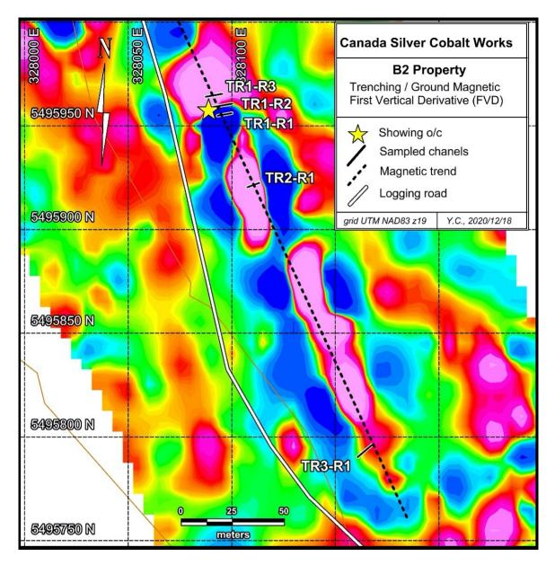
Figure 3. B2 Showing and channel location with ground geophysical survey
