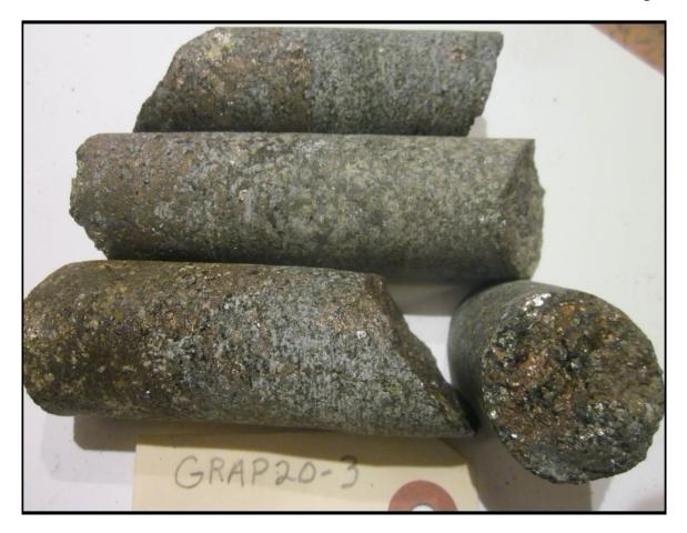
Figure 4 (3.2cm-diameter Core) Sulphide mineralization in Verification Core of Grand Portage showing
